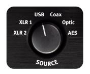
Use the Source switch to select an analog or digital input source.
