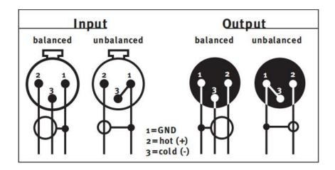
Connections to RCA sockets are always unbalanced, a wiring to jack connectors can be both balanced (1/4" TRS/stereo jack) or unbalanced (1/4" TS/mono jack). We recommend to use individually configured cables from XLR to RCA or jack sockets instead of adaptors. You can get cables in any needed configuration from audio dealers. With the diagram above, the dealer can ensure to provide the appropriate cable for your application.
