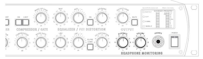
An individual monitoring mix is important for best working conditions and especially a good intonation. That is why the Channel One is equipped with a headphone monitor section, providing a headphone amplifier and a mixing stage to generate an individual mix for the musician with playback and recording signals.
