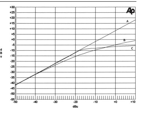
Diagram 2 shows various cut and boost settings of the air band filter.
