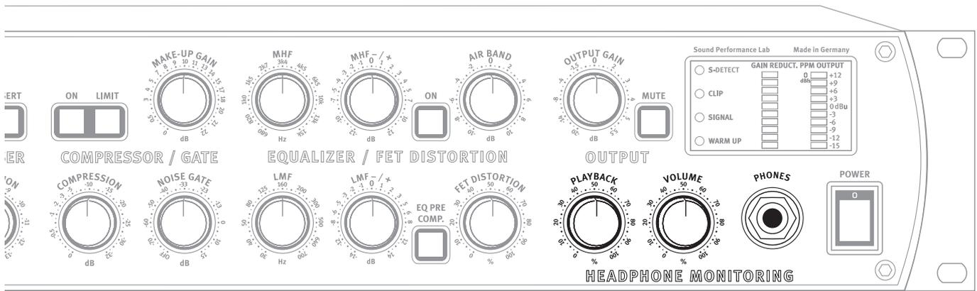
An individual monitoring mix is important for best working conditions and especially a good intonation. That is why the Channel One is equipped with a headphone monitor section, providing a headphone amplifier and a mixing stage to generate an individual mix for the musician with playback and recording signals.
