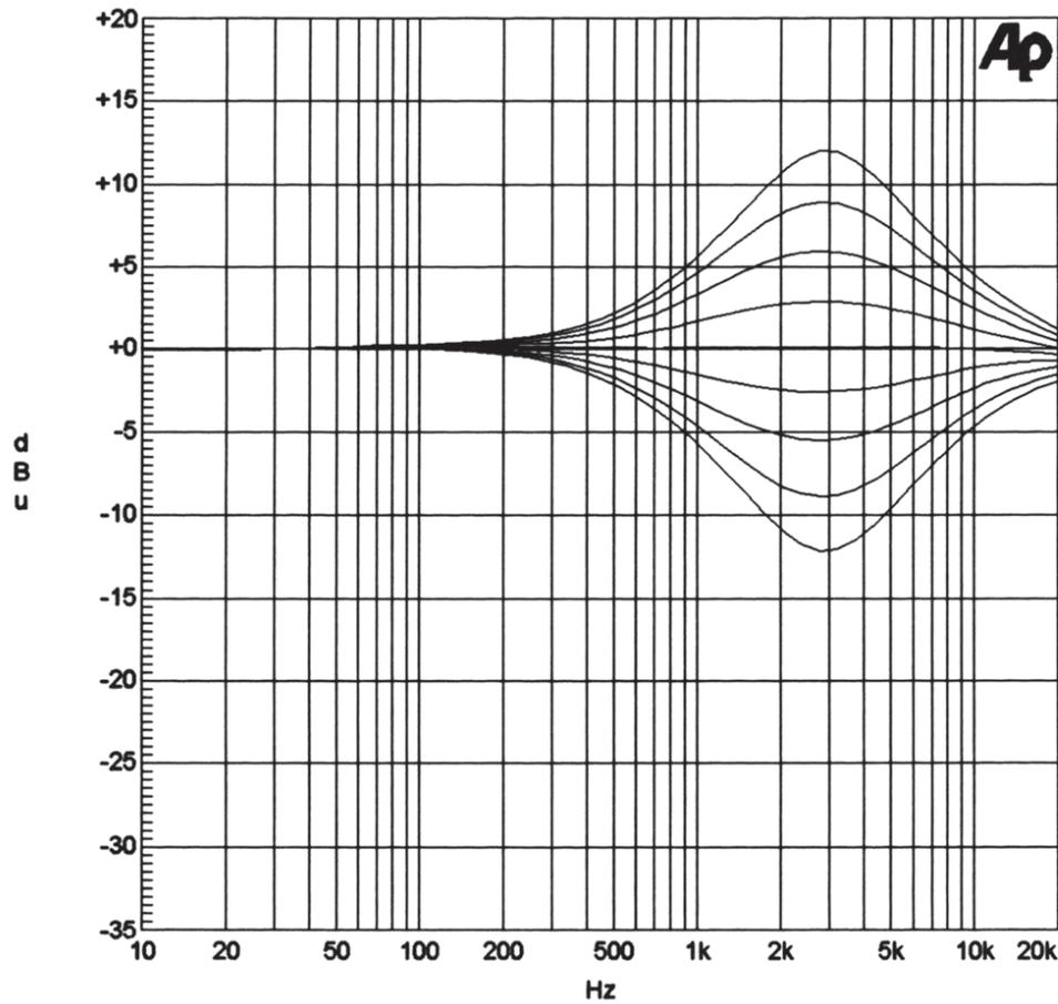
Diagram 3 displays various cut and boost settings of the MHF filter at 3 kHz.
