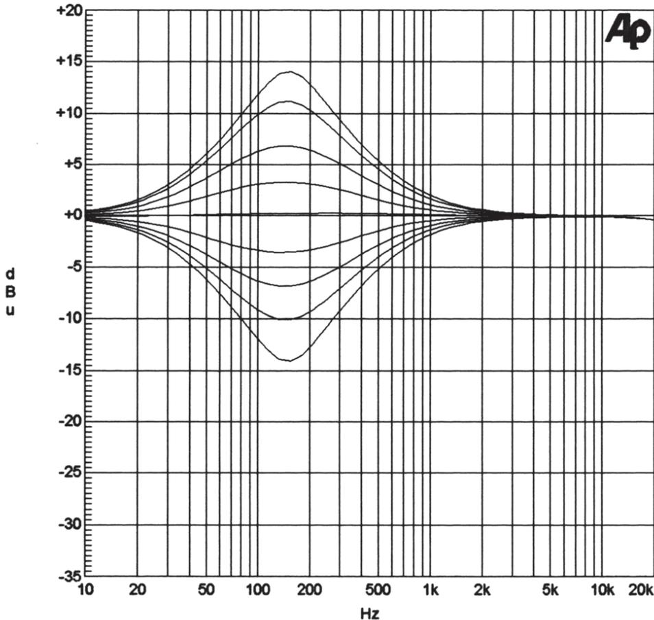
Diagram 4 displays the curves of the LMF filter.
