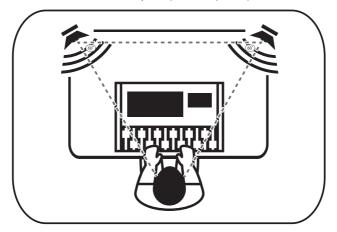
The speakers should be separated so that the AMT tweeters form an equilateral triangle with your head. The monitors should be "toed in," or angled, so that they are pointed at you, not pointed straight ahead.
