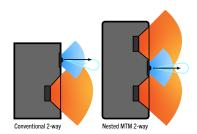
Conventional 2-way speaker designs can cause significant early reflections from their surrounding environment. The Eris E44 studio monitor overcomes this by positioning a 1.25-inch, silk dome
