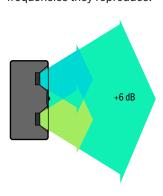
The combined signal of the two relatively small drivers propagates forward like a single waveform, behaving like a single, larger driver. This mutual coupling provides a highly dynamic output in a compact footprint. At the same time, the two smaller woofers work in parallel to partially contain the dispersion of the tweeter, minimizing phase
