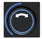
**Illuminated Knob Position -** The illuminated ring around the knob shows relative knob position and changes color depending on the active mode. It shows the current relative position of the knob for either main output, gain, or headphone level.
