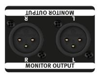
The Monitor output is electronically balanced and implemented via XLR connectors. The Monitor Output is connected in parallel to the Master Output and provides the stereo mix for a monitor controller or a pair of studio monitoring speakers.
